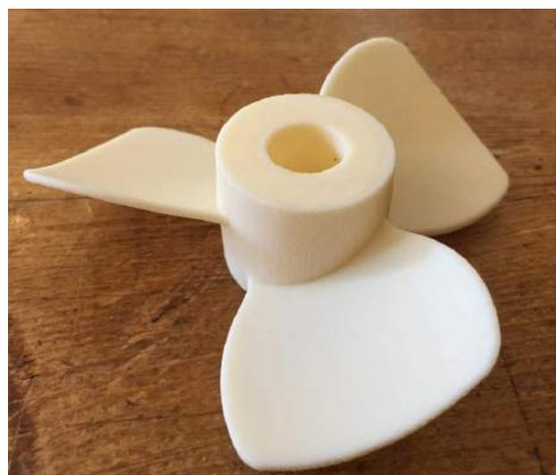
From there all that is to be done is to let the machine do its thing; the build process is mostly automatic. Each layer is usually about 0.1 mm thick, though it can be much thinner or thicker. Depending on the object's size, the machine and the materials used, this process could take hours or even days to complete. The machine is periodically checked to make sure there are no errors.
